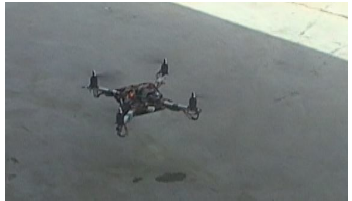
Figure 3. Second version of the Quadbobber lifting a square wooden block of 140g as payload. There was no change in the control efficiency of the craft.
