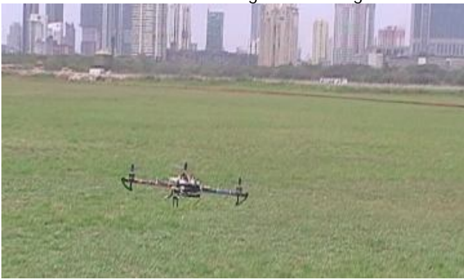
Figure 1. The DCM algorithm being tested on a commercial frame. This flight showed that sensor orientation can change in flight and still provide very good control.
